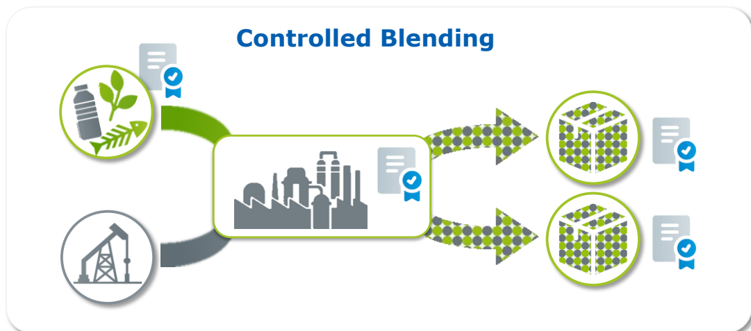
Figure 4: Diagram representing a controlled-blending process. Incoming sustainable and conventional materials are processed together, mixed in known proportions, with the result that all products contain the same physical proportion of sustainable materials.
